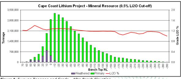
Figure 1: Ewoyaa Tonnage and Grade - 10m Bench Elevation
