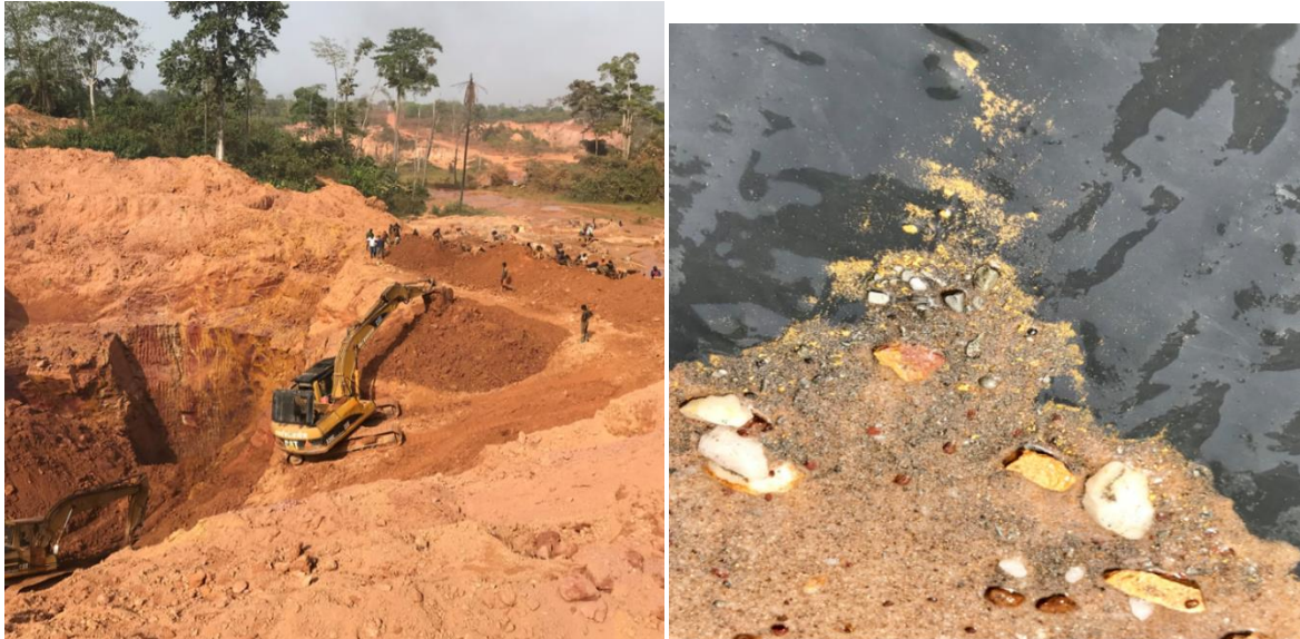
Figure 6: Artisanal workings within the license area and visible gold observed in a washing pan.
