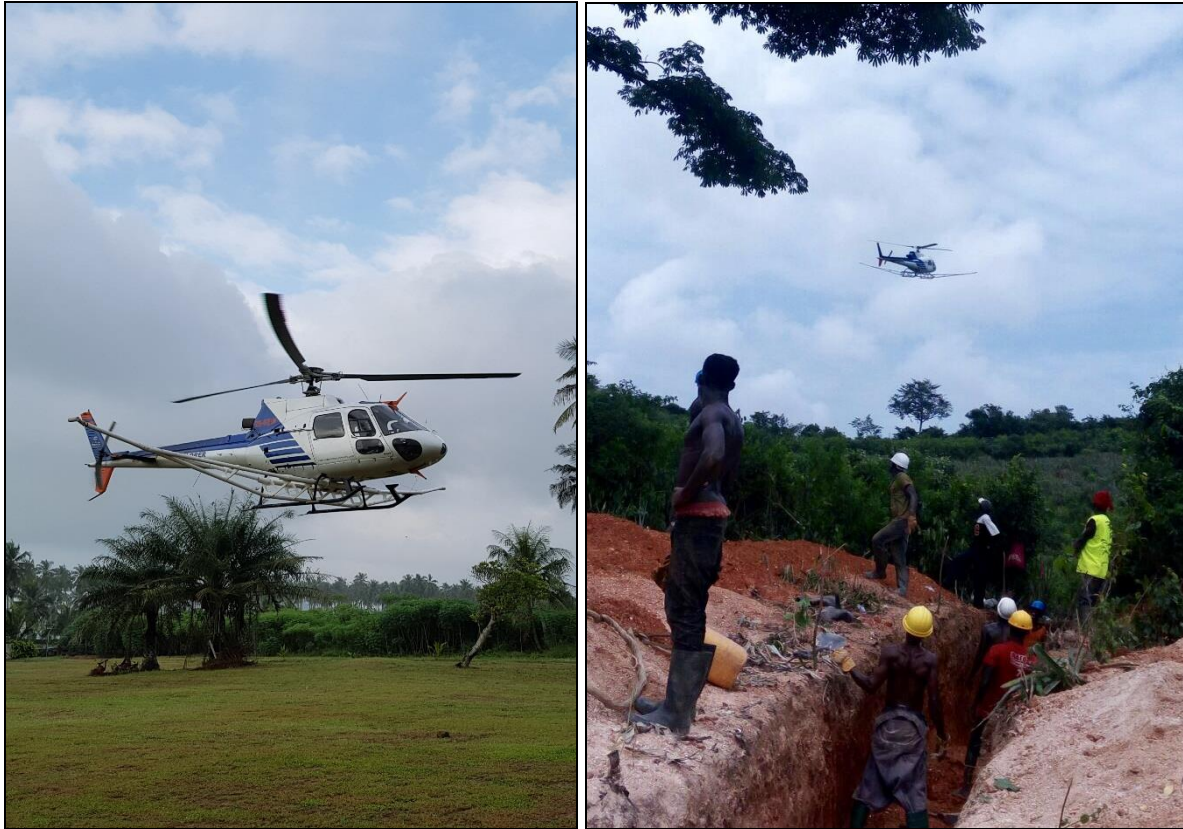
Figure 8: New Resolution Geophysics (NRG) helicopter with geophysical equipment taking off from Cape Coast base and (right) trenching underway at the Ewoyaa prospect with light coloured spodumene bearing pegmatite in the trench.
