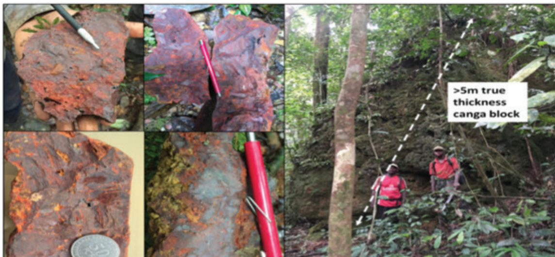
Figure 4: DSO/near DSO canga mineralisation sampled within the Mt Pele area showing massive, low porosity, hematite-goethite replacement of clasts and matrix (left), and rotated canga block along margin of canga plateau showing potential >5m thickness of canga mineralisation.
